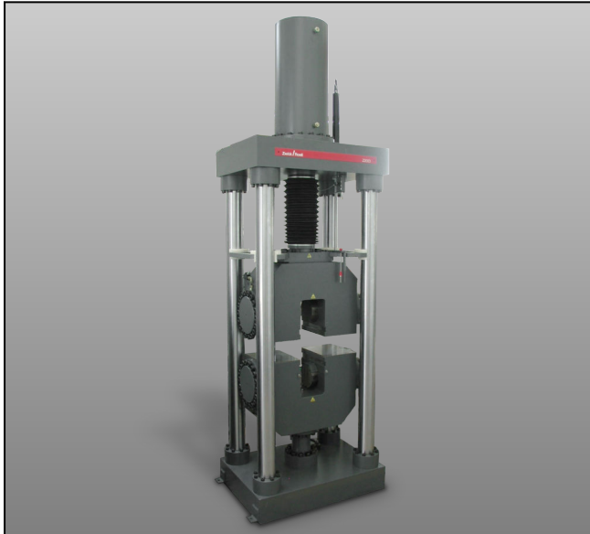
ZwickRoell Z2000H with hydraulic grips
